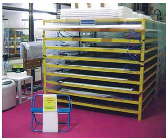
Figure shows assembly and testing infrastructure at NPD-BARC. The lab has an associated storage area and is backed by a robust workshop for handling all the relevant mechanical jobs. The HV, LV, 4 channel gas mixing unit, 8 channel gas flow system and gas recovery unit are fully operational. The cosmic ray stand can handle eight RPCs of RE*/3 type at a time. Scintillators of the relevant sizes are under fabrication at BARC, Centre for Design and Manufacture and accordingly the cosmic hodoscope would be set up to study the chamber.
